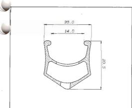
Contax has been designed for the most demanding competition. It's compact cross section design and light weight make it ideal for racing applications.
